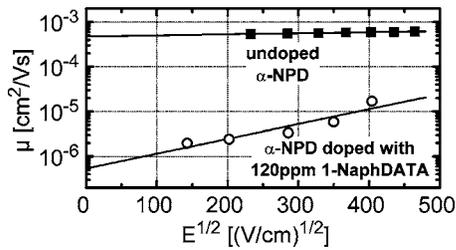
FIG. 2. Hole mobility  $\mu$  for undoped  $\alpha$ -NPD and  $\alpha$ -NPD doped with 120 ppm 1-NaphDATA vs  $\sqrt{E}$ . The straight lines and fits according to Eq. (2).
