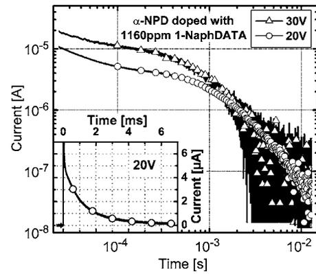
FIG. 3. Hole current transients for  $\alpha$ -NPD doped with 1160 ppm 1-NaphDATA for two applied voltages in double logarithmic scale. The inset exemplarily shows one transient in linear scale.
