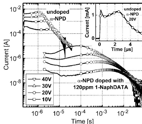
FIG. 1. Hole current transients for undoped  $\alpha$ -NPD and  $\alpha$ -NPD doped with 120 ppm 1-NaphDATA for various applied voltages in a double logarithmic plot. The inset exemplarily shows one transient in linear scale.
